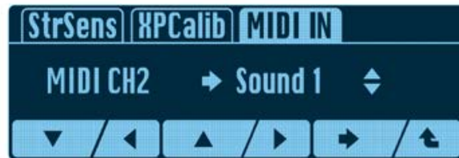
Press the 'patch +' switch multiple times until 'Sound 1' is displayed.
