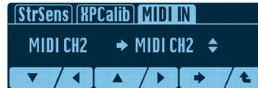
Press-and-hold 'patch +' switch to move selector arrows to the new destination channel
