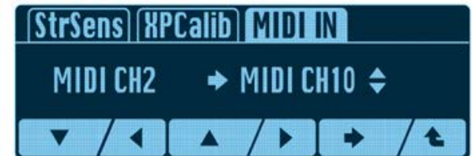
Press the 'patch +' switch to set the destination MIDI channel to MIDI channel 10
