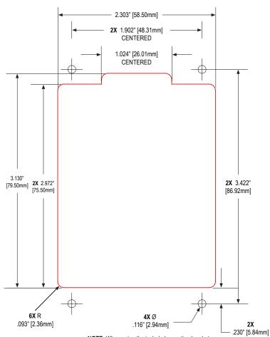
**NOTE:** When using the included mounting brackets, screw holes should be .116" [2.94mm] as shown.
