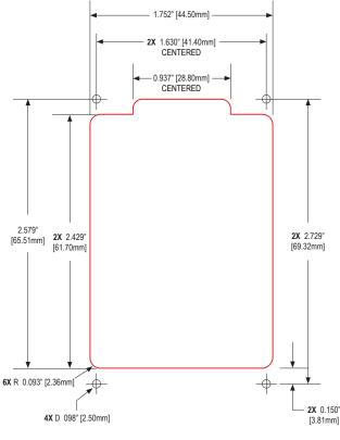
NOTE: When using the included mounting brackets, screw holes should be .098" [2.50mm] as shown. When not using the included mounting bracket, drill an appropriately sized pilot hole.
